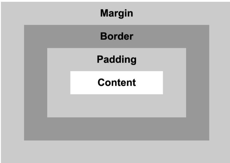
FIGURE 5.1 The mighty box model. At the center is the content itself. Surrounding that is the padding. Surrounding that is the border and surrounding that is the margin.
