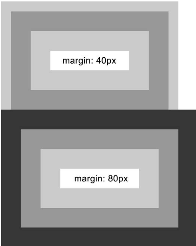
FIGURE 5.7 “Margin collapsing”: When two vertical margins come into contact, only one will apply.
