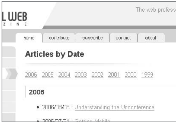
FIGURE 6.8 Digital Web's site-wide primary navigation and the years depicted at the top of this page are unordered and ordered lists, respectively. The primary navigation (the tabs) is made up of list items set to float left. The list of years comprises list items set to display inline.
