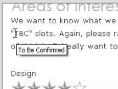
FIGURE 2.4 All hail the tool tip! If an abbreviation has a title attribute, its value can be used to state the full phrase that the abbreviation represents.
