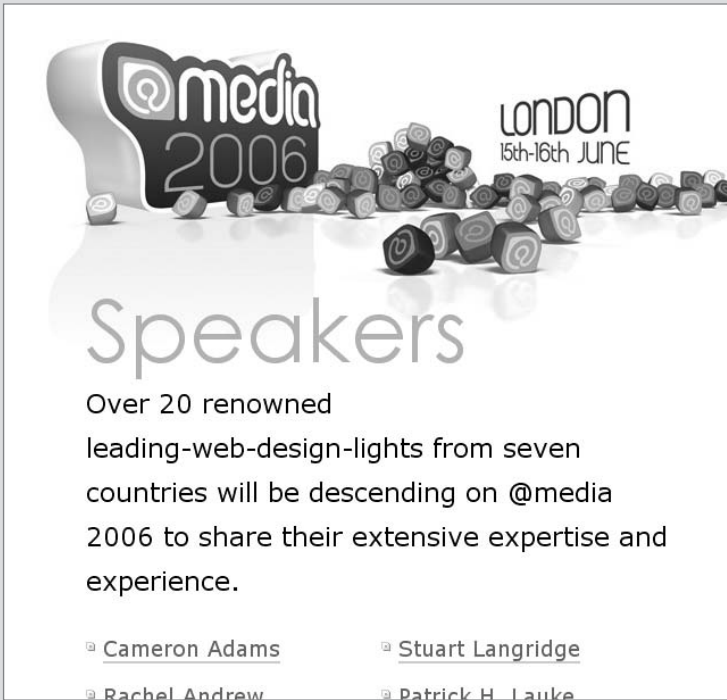
FIGURE 2.7 Because the font sizes are all set in ems (after an initial setting in percentages), users can bump up the size of the text, if they so choose, which is a great accessibility benefit. If they were set in pixels, the majority of web surfers, using IE, would not have this benefit.
