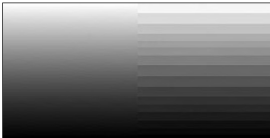
Figure 7.3 The left shows a 32-bit rendering of a color gradient, and the right shows a banded 15-bit rendering of a color gradient.
