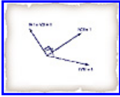
Figure E-20 Calculating the normal of a plane
