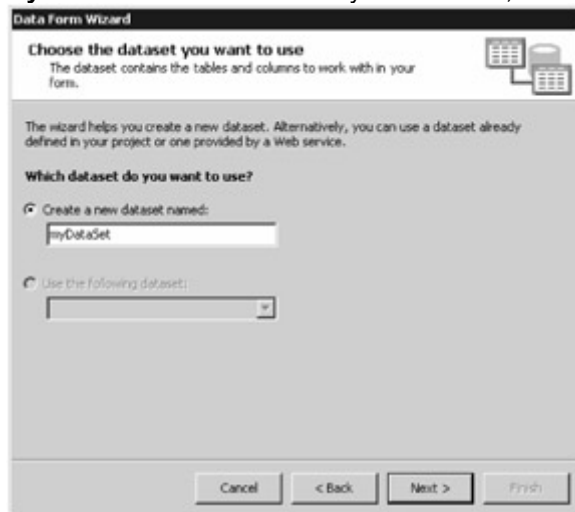
Figure 6.19: Entering the name of the new DataSet Click the Next button to go to the next step.
