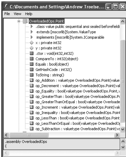
Figure 9-1. In terms of CIL, overloaded operators map to hidden methods.
