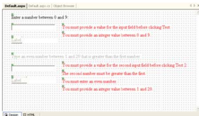
Figure 15.2: Using validators means setting aside space for text that might never appear on screen.
