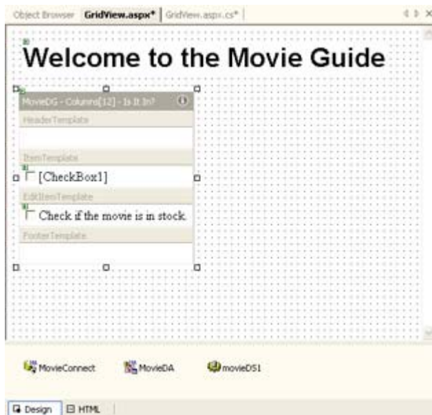
Figure 15.7: The template-editing window enables you to add new template functionality by dragging and dropping controls.
