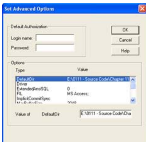
Figure 11.4: The Set Advanced Options dialog box includes features such as the login name and password.
