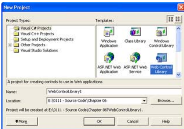
Figure 6.13: Use the New Project dialog box to select the Web Control Library template.
