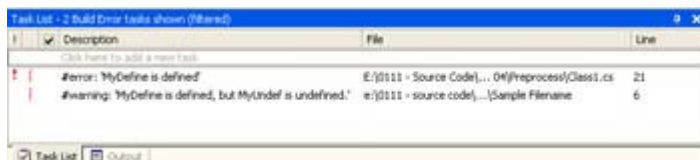
Figure 4.5: The #warning and #error directives provide output you can use as a reminder.
